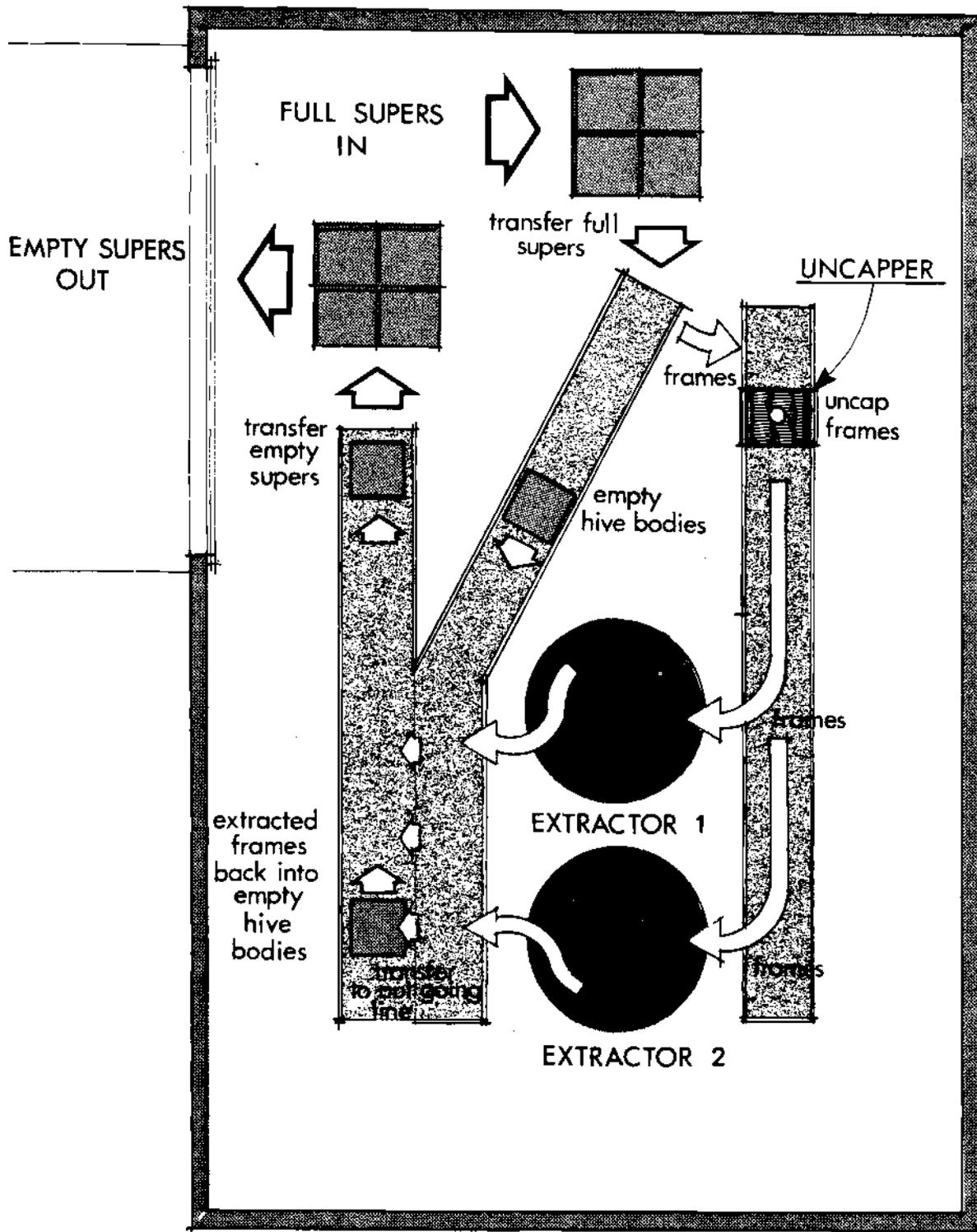
FIGURE 4: U-FLOW FOR VERTICAL AXIS EXTRACTOR USING CONVEYORS
