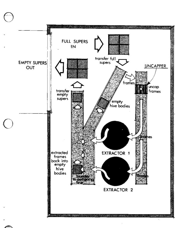
FIGURE 4: U-FLOW FOR VERTICAL AXIS EXTRACTOR USING CONVEYORS
