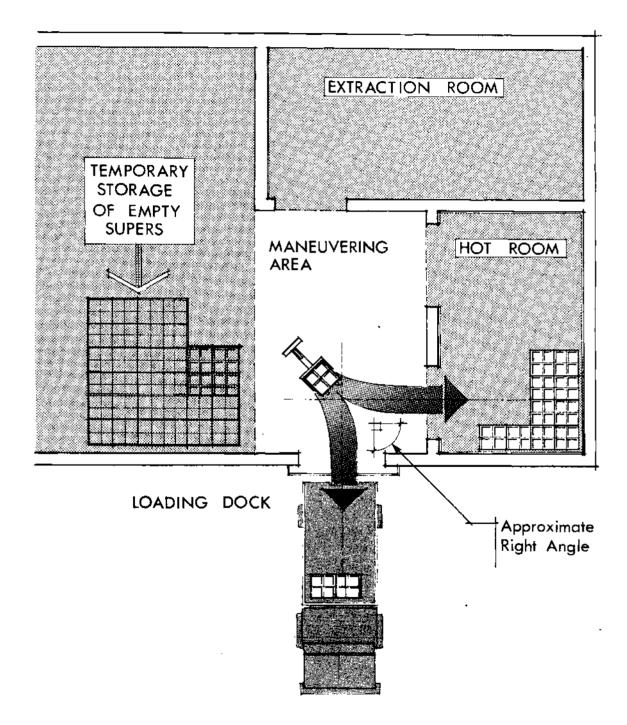
FIGURE 7: ILLUSTRATION OF THE RIGHT ANGLE PRINCIPLE
