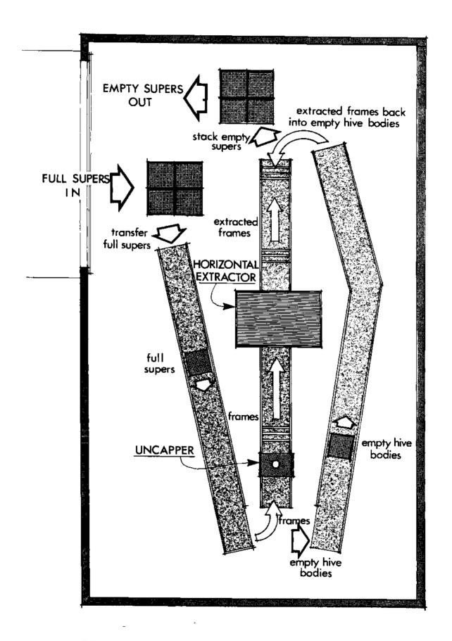
FIGURE 5: U-FLOW FOR HORIZONTAL EXTRACTOR USING CONVEYORS
